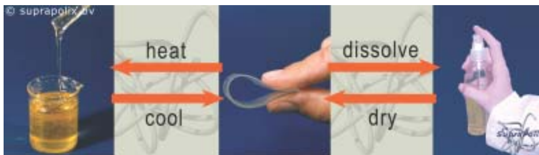
Fig. 3 Illustration of the phase changes in a rubbery material based on Kraton®, (poly(ethylene-co-butylene), modified with UPy, exemplifying the diversity in phase behavior because of the supramolecular interactions. (Reproduced with permission of SupraPolix BV.)
